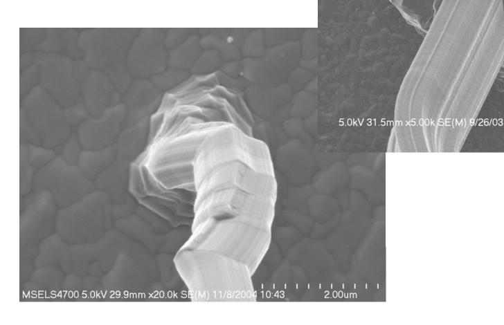
Odd shaped eruption (OSE) on 15 um thick Sn-3wt%Cu electrodeposit on phosphor bronze substrate
